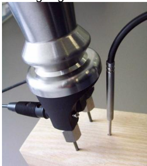
Reciprocating piston electrode GHE91 with temperature-probe GTF38
