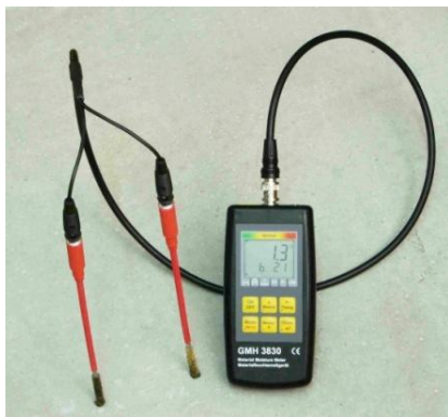
Measuring with brush probe GBSL91
